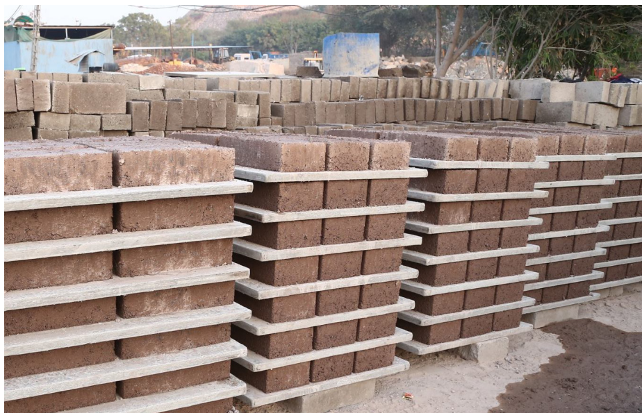
Figure 15: Paver Bricks from recycled material at Burari Site
